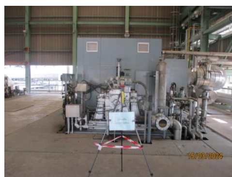
Propylene Compressor (R-650)
